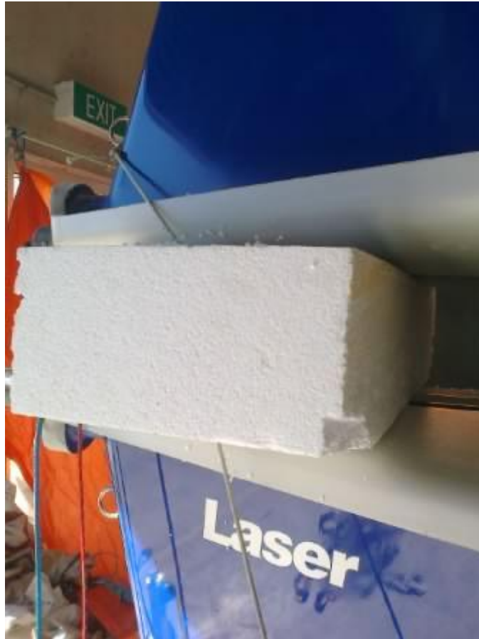
Figure 6 - Bow block with locator/safety tie to trailer/boat
