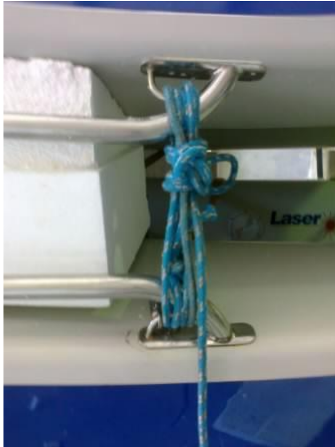
Figure 7 - Tie boats together firmly
