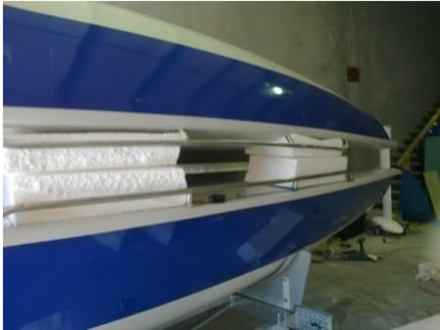
Figure 4 - Wedge blocks in situ (note please tape them together - we didn't)
